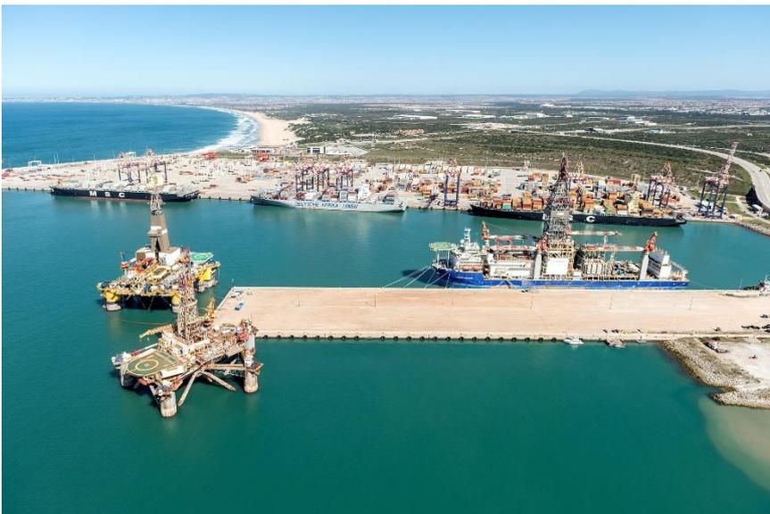
Pilot Ziggy Duwe positioned all three these vessels alongside this berth in the Port of Ngqura. Merely the look of the two oil rigs (left) gives one an idea of the complexity of tug handling required to position them – they also have no propulsion units, which contribute to the complexity. The drill ship (right) has six propulsion units – therefore it is a lot easier to manoeuvre.
