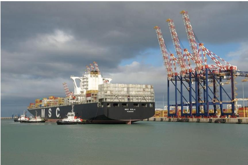
A typical manoeuvre of tugs pushing the vessel alongside the quay.
